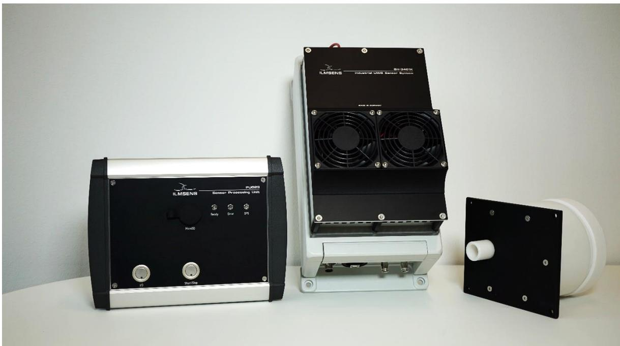
*Figure 1: Layer thickness measurement system consisting of (from left to right) a control panel connected to the layer thickness sensor module via an interconnection cable and two antennas connected to the sensor via two coaxial-cables.*
